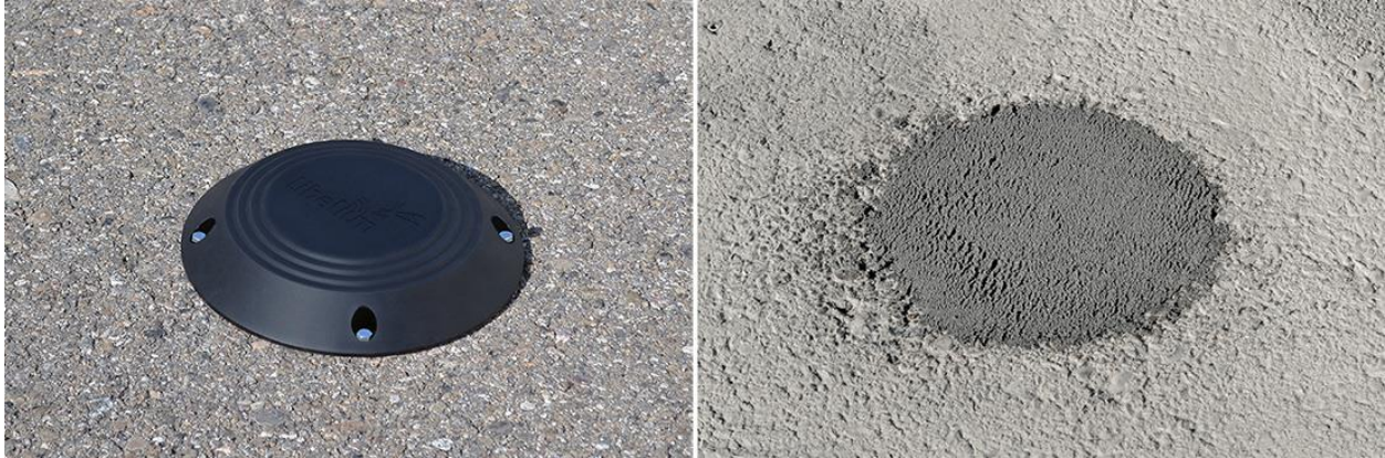
Figure 4.6 Installation methods of IoT sensors: same sensor, installed on the surface or fully sunken
