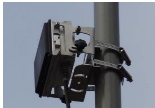
Joonis 1.1 Smartmicro UMRR-12 radar
